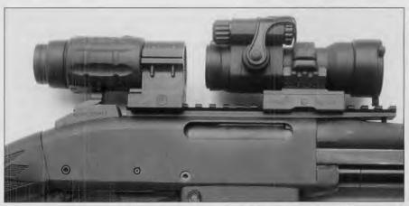
Aimpoint's brand new QD 3X Extender was tested on the 7615P along with the Aimpoint Comp ML2 Red Dot Sight. (right) To remove the 3X Extender for CQB, simply unlock, twist 90 degrees and lift off/replace with no effect on zero. The combination is seen here on MSP's MOA Solution M1913 extended rail.
